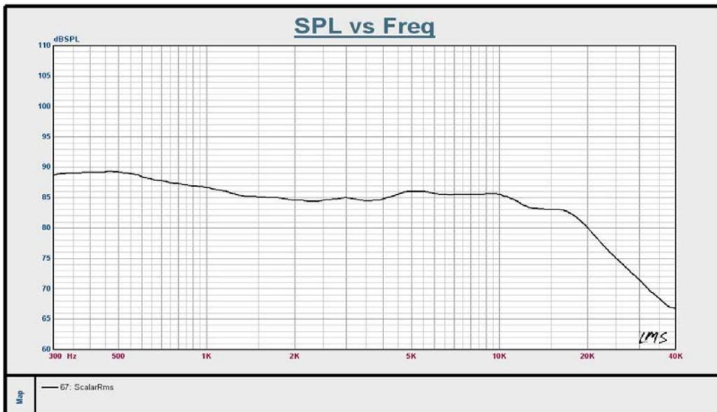
Figure 4 - MTM Center Channel Power Response
